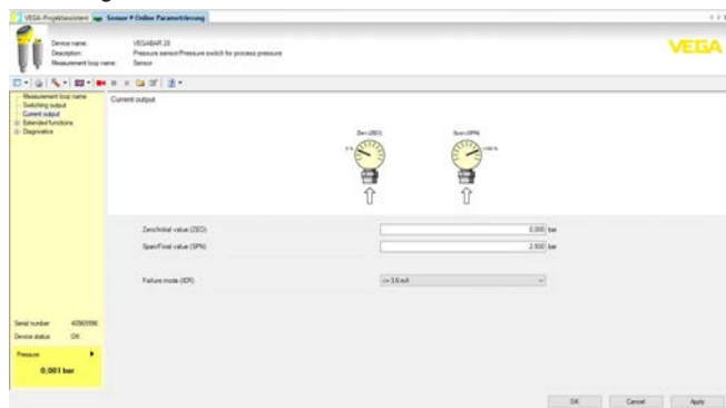
Fig. 24: Example of a DTM view - Adjustment current output
