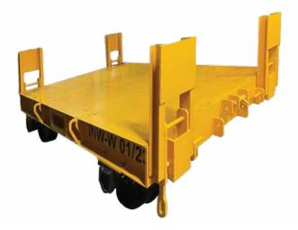
The use of electric motors ensures autonomous movement without rolling stock. The bogie is delivered to the testing site by road carriage and then travels to the target measuring location by itself, using the installed drive. The advantage of this solution is independence from the locomotive.
