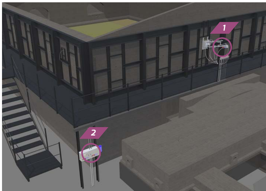
THE NIR-B MONITOR ON THE TANK WALL (1) WITH THE CONTROL BOX SITUATED FURTHER AWAY (2)
