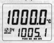
③ Press "MX/MN" key for 2 seconds to exit MX/MN mode. In MX/MN mode, the "C/F/K" and "TYPE" key are not active.
