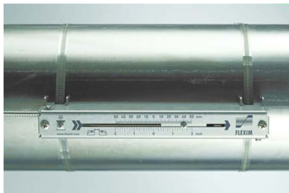
Measurement with transducers mounted by Variofix L
