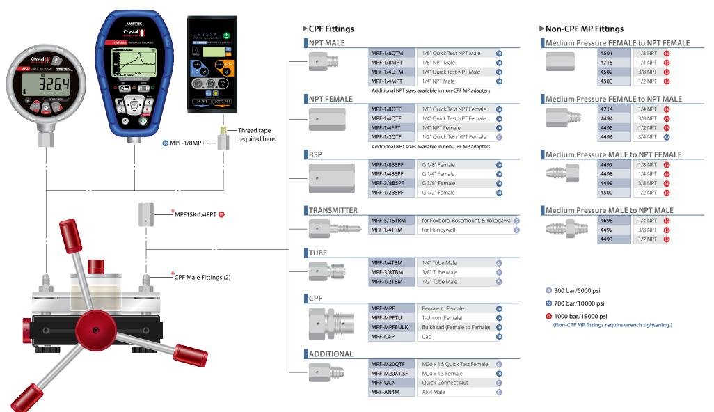
\*These parts are included with the pump. All other parts are supplied as part of a pump system, or may be ordered separately. All BSP connections require bonded seals.
